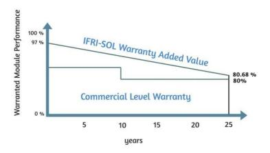
For Mono crystalline Products: less than 3 % in the first year, thereafter less than 0.68 % per year, ending with no less than 80.68 % in the 25th year after the Warranty Start Date.
